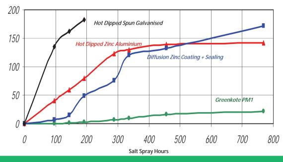
Failure is reached when the area of substrate corrosion exceeds 5% of the total sample area.
