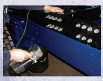
Smaller diameters used in the truck and trailer industry clearly demonstrate the anti vibration qualities of TCBs
