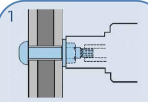
The inner socket of the shear wrench fits over the bolts spline while the outer socket fits over the nut.
