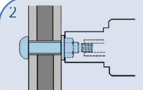
Press the trigger switch. The outer socket rotates clockwise and tightens the nut. When the correct preload is reached the outer socket stops rotating, the inner socket counter rotates and shears the spline off.
