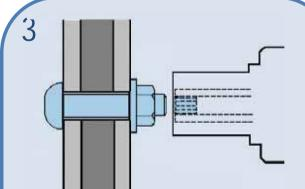
Stop the wrench and pull the outer socket off the nut. The spline is retained in the inner socket.
