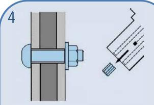
The wrench has a second trigger to eject the spline safely. The bolt is now properly installed with the correct tension.
