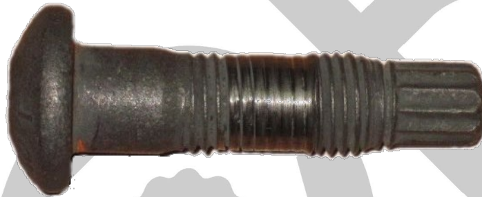
Example of thread stripping
