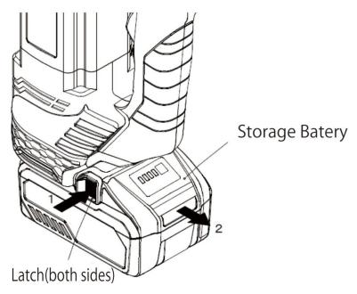
When attaching a battery pack to the wrench body, align the grooves on the battery pack with the grooves on the wrench body and insert completely until you hear a click.
