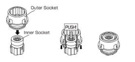
Set inner & outer socket assembly to the wrench body and completely remove the gap between socket assembly and wrench body. The gap can be removed by turning & pushing down screwdriver or TC bolt into the inner socket.
